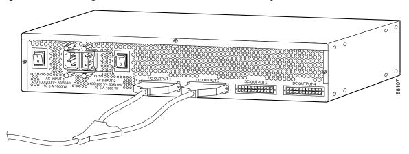
Step 4 On the Cisco RPS rear panel, connect one or two AC power cables. A single AC power cable can go into either AC connector. Two AC power cables provide parallel AC power sources. Use the cable locks on the Cisco RPS to lock the cables in place. (See Figure 16.)
